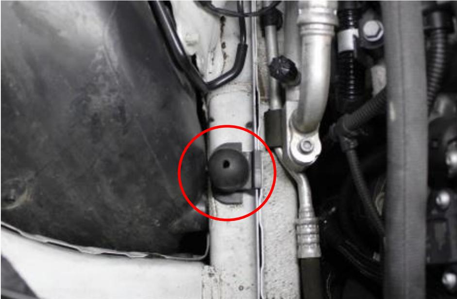
9. Remove the rubber mounts which cushion the stock airboxes. These can just be pulled out. Keep them aside – they are required shortly.
