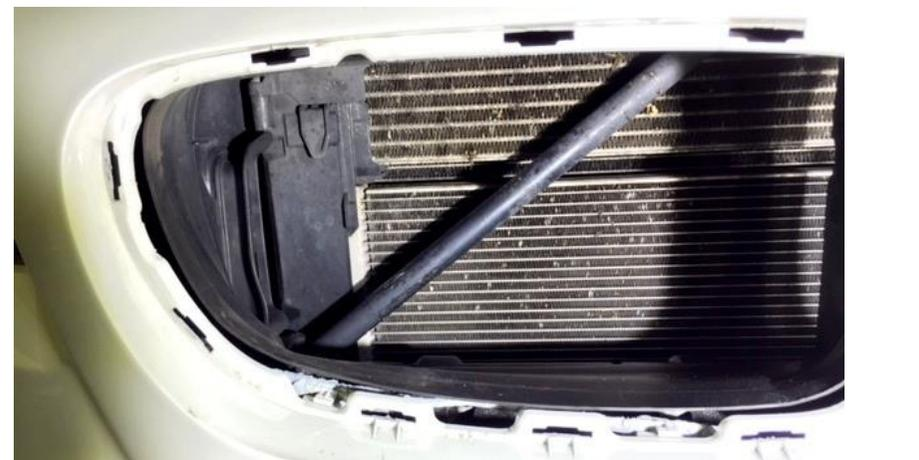
35. Starting with the LHS Scoop – look into the left side of the bumper. The clips on the back of the scoop will secure onto this strut brace.
