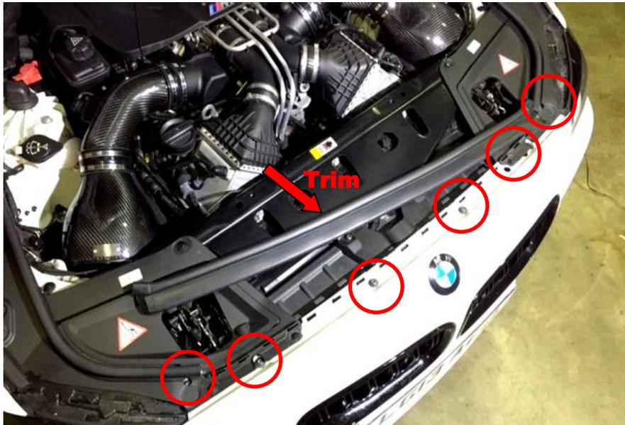
32. We will now install the scoops. To remove the nose grills, you need access to the grill clips. Start by pulling the rubber trim off the top of the bumper cover. Then remove the Torx screws and plastic clips securing the top of the bumper cover.
