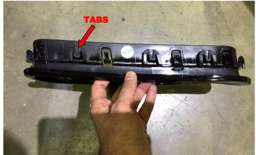
33. Pull the bumper cover out to gain access to the top of the grills. You will see tabs which need to be pushed in using a screwdriver. Pull the grills out while pushing these tabs in. You can pull the bottom tabs up with your fingers.
