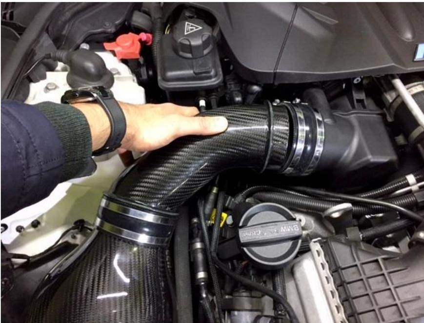
26. Now turn the Carbon tube downwards and into the silicon coupler as shown. Loosen the hose clamp around the silicon if required.
