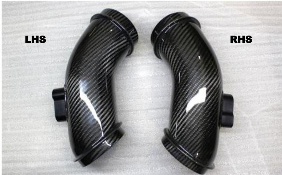
21. Identify the LHS and RHS Carbon inlet tubes as shown. The MAF sensor mounts are closer to the bottom of each tube.
