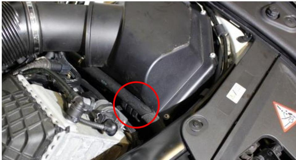
3. Remove the rubber hose from the airbox clamp and move out of the way.
