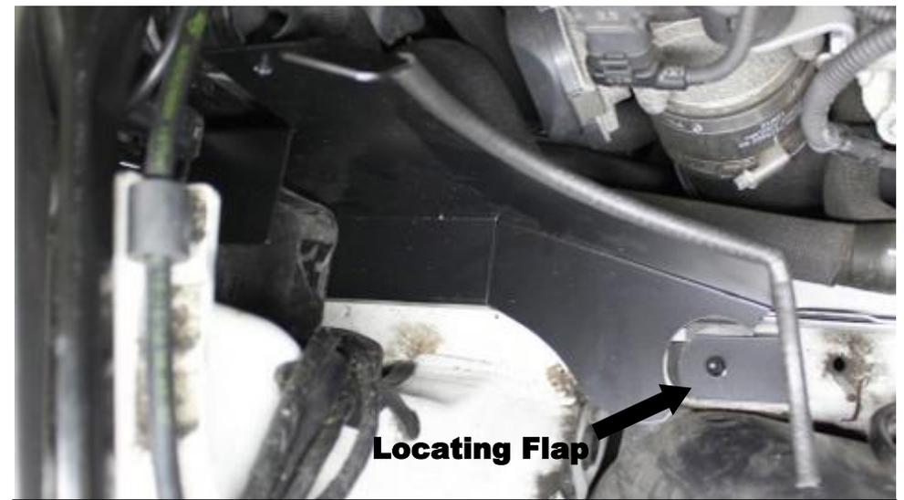
16. Push the shield towards the front of the car until the hole in the locating flap lines up with the plastic stud which the rubber grommet was removed from in step 9. Push the flap down into the stud.
