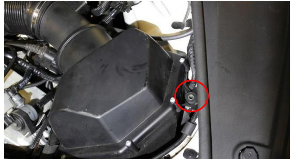
2. Starting from the right hand side remove the Torx screw securing the airbox in place as shown.
