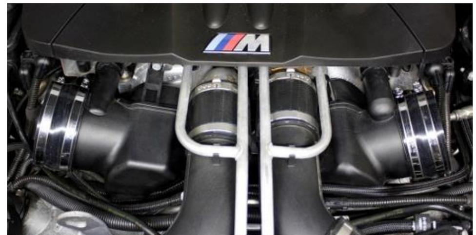
20. Push the 83mm silicon couplers over the turbo inlets as shown. Push them on fully and tighten the first hose clamps on both sides to secure to the inlets. Ensure the clamps are straight. Leave the outer clamps loose.
