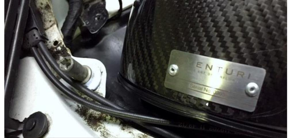
28. There should be adequate clearance between the housing and the front panel. Since the clamps are still loose – you can rotate the tube and the housing until you have good clearance.
