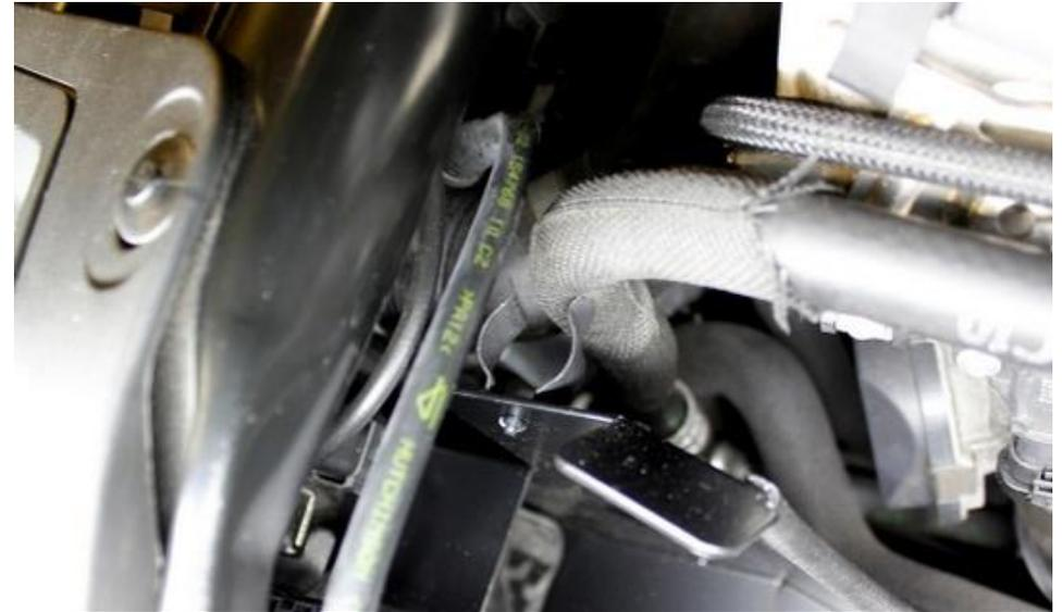
18. Finally secure the stock rubber hose into the clip on the side of the shield. Repeat this process from step 14 for the other side.
