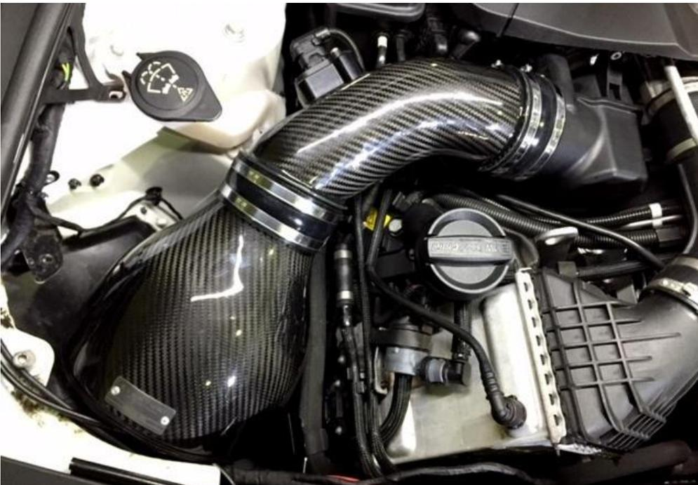
29. The MAF sensor mount should be at the back of the tube as shown – insert the MAF plug back into the sensor. Push it in fully. Now tighten all the hose clamps. Ensure the housing is pushed up into the tube fully and the tube is pushed into the turbo inlet fully.
