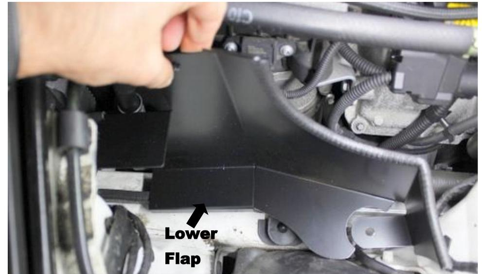
14. Starting with the RHS shield, place it in the right hand cavity, position the lower flap over the rubber edging previously inserted.
