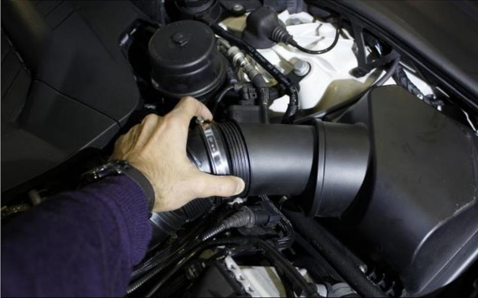
5. Loosen hose clamp around the airbox and pull the plastic inlet tube off the airbox.
